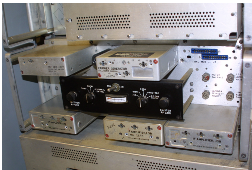
Figure 2. SSB Generator Chassis with the Balanced Modulator Module Removed
