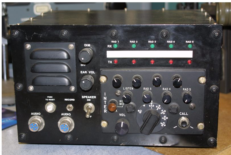
Figure 4. AN/AIC-25 Interphone Control
