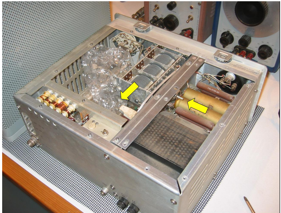
Figure 3. Covers off and HV Shorting Switches, Or Interlocks Annotated
